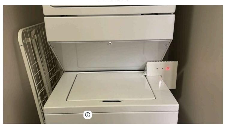
The Laundry Detector checks to see if laundry is done at any given moment. It has three inputs: time, distanc and acceleration. These three factors into the open state of the laundry door, the movement of the machine itsen, and how long it has been since it last moved.
