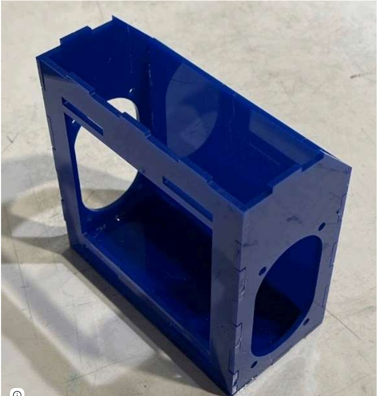
Glued pieces of laser cut acrylic
